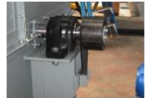
Typical Head Bearing Assembly & Anti Roll Back
