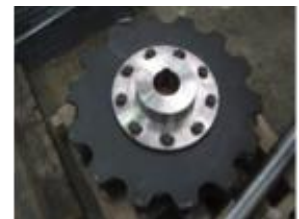
Typical Segmented Chain Wheel Sprocket
